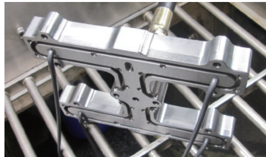
分流板流道拋光 Polishing of Manifold Runners
